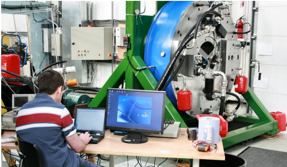
Figure 4.3. 1 MN-m hydraulic wind turbine transmission under test
