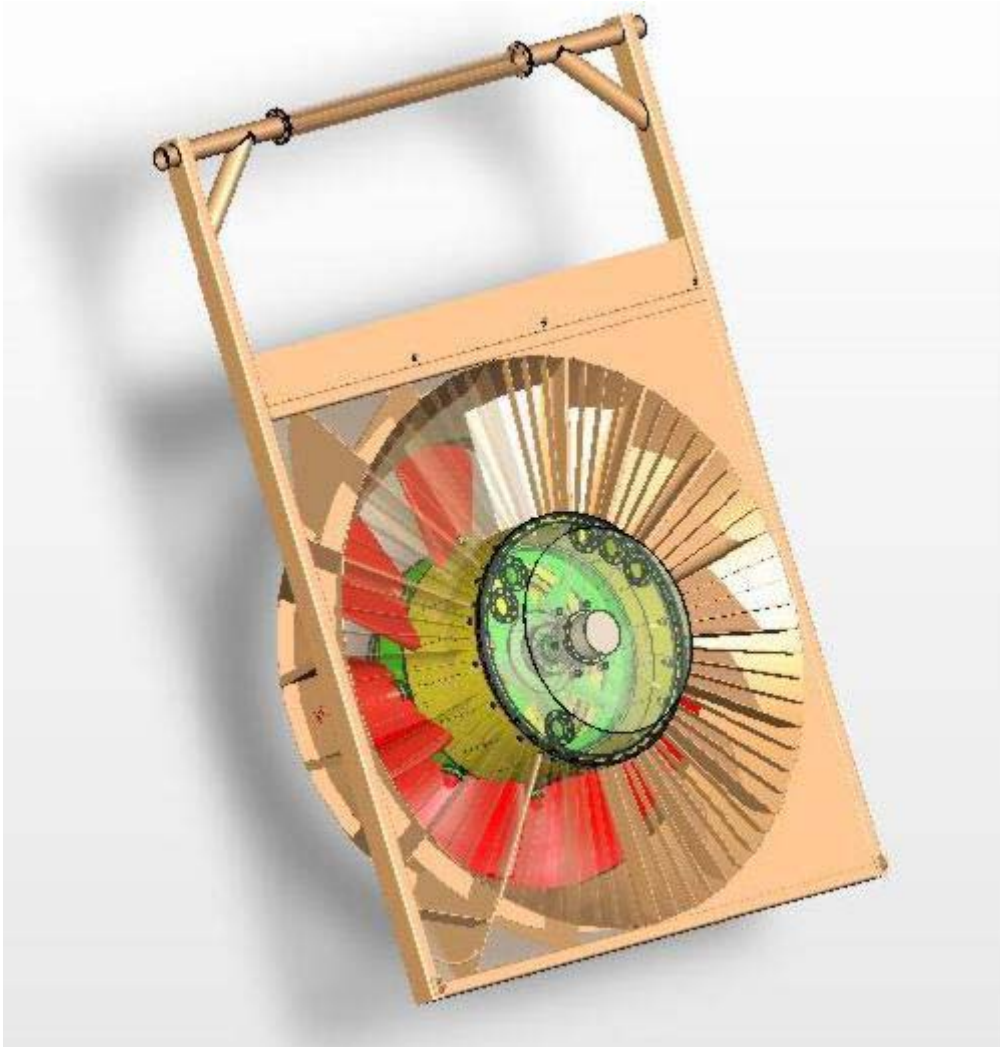
Figure 4.2. Internal structure of MJ2 turbine
